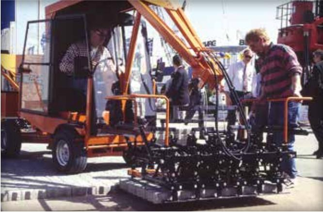
Figure 3. Motorized equipment with a mechanical clamp.
